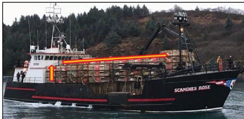
Figure 30 – Arrows indicate the general route a crewmember would have to take to climb up to the top of the pot stack and then go forward to do a full assessment of the ice accumulation on the accident voyage. (Source CG Exhibit 014, with markups)
