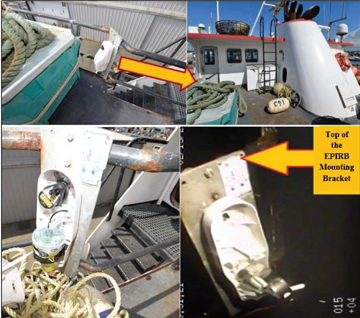
Figure 44 – Composite of photomontage of the SCANDIES ROSE EPIRB. Top left, EPIRB in housing on the inside of top rail aft of the wheelhouse. Top, right is the location shown with the yellow arrow in reference to the position in relationship to the port wheelhouse door. Bottom left, the open EPIRB housing during inspection for 2019 Valuation and Condition Survey. Bottom right, the empty housing as seen during underwater ROV site survey February 2020. (Source – [REDACTED] photos for 2019 Valuation Survey and bottom right, CG Exhibit 008)
