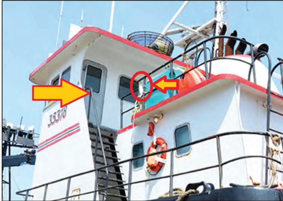
Figure 13 – Large arrow points to the port side wheelhouse door on the SCANDIES ROSE. The smaller arrow points to the location where the EPIRB was stored in the float free bracket, which is circled in red. (Source CG Exhibit 004, with markup)
