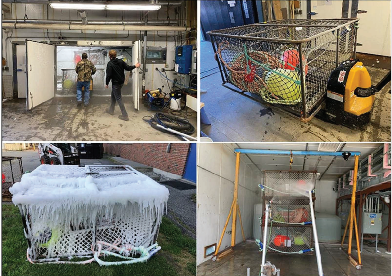
Figure 109 – Testing at the CRREL facility in Hanover, NH in September 2021. In this composite of testing photos, top left two technicians enter the smaller of the two test chambers to set up for two vertical pot stack testing. Top right one of the pots with the associated gear being maneuvered into the test chamber. Lower, left a single pot after removal from the chamber showing the formation of ice on the single pot. Lower right inside the larger chamber with a triple pot stack hanging from the load cell. In the foreground are the two oscillating sprayers directing saltwater spray onto the triple pot stack based on the configuration requirements in the test plan matrix of tests. (Source Coast Guard)
