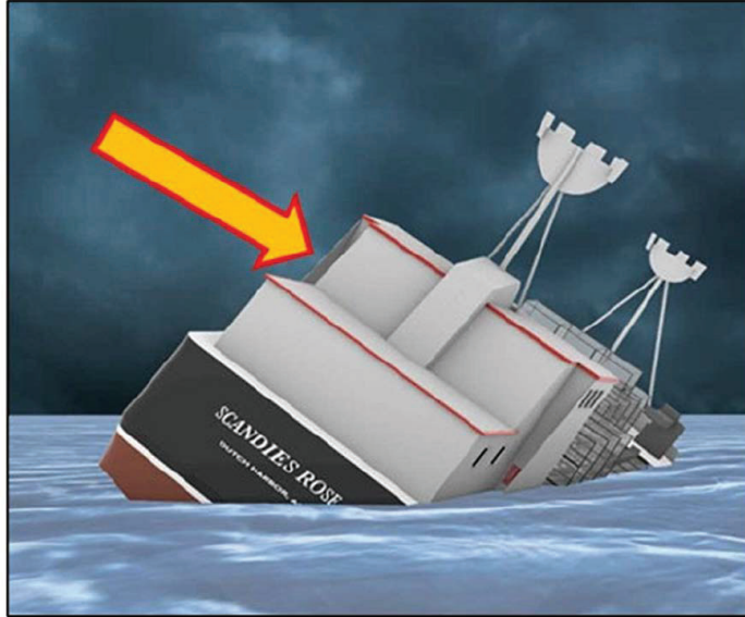
Figure 15 – Yellow arrow points to the approximate location of the survivors when they exited the SCANDIES ROSE wheelhouse port side door. They later moved forward as the vessel began to sink and a wave washed them overboard. The MSC model is displaying an approximate list to starboard of 35 degrees. (Source Coast Guard)
