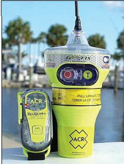
Figure 104 – On the left, is an ACR Electronics Inc. version of a PLB that could have been carried by the crewmembers on the vessel. On the right of the same image is an EPIRB of the type and manufacture that was carried on the SCANDIES ROSE. The figure gives a perspective as to the size of the devices in comparison to one another. (Source Coast Guard)
