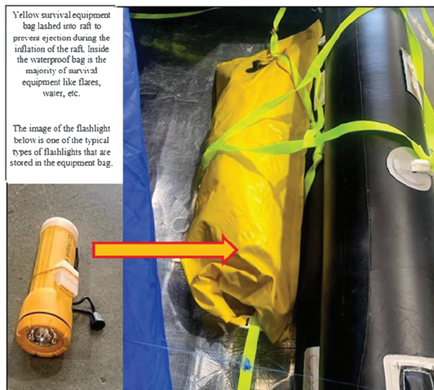
Figure 99 – Image showing the raft equipment bag, indicated by the yellow arrow that is lashed to the floor of the raft near the boarding area. On the left side of the figure there is an example of a D-cell flashlight stored in an equipment bag. (Source Marine Safety Services, Inc.)
