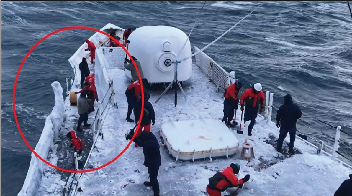
Figure 22 – Image of USCGC MELLON crewmembers on the bow of the vessel breaking ice shortly after arriving in the search area. The red circle shows the difference between a de-iced portion of the port side railing and the parts of the ship that had not yet been de-iced highlighting the level of ice accretion the CGC MELLON experienced as it steamed to the SCANDIES ROSE's last known position. (Source Coast Guard Exhibit 095 screen capture, with markups)
