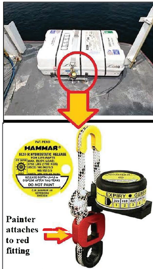
Figure 45 – One of two liferafts on the SCANDIES ROSE. Circled in red is the hydrostatic release device which allows the liferaft to inflate and float free of the vessel as it sank. The close-up of the hydrostatic release device shows the point where the liferaft painter attaches, once the device activates, the raft floats free, inflates and then the painter is released from the device allowing the raft to stay on the surface. (Source CG Exhibit 004 and close-up from the CG D17 Commercial Fishing Vessel Safety Reference Guide http://www.fishsafewest.info/PDFs/D17CFVSE_JobAid.pdf )
