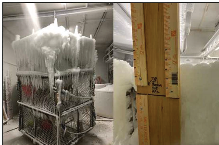
Figure 97 – These images demonstrate the difficulty in determining the thickness of ice in crab pots being subjected to freezing spray in a -15° F chamber during the ice accretion testing in September 2021. Left, a three pot stack with a significant accumulation of ice. Right, a ruler that is used to accurately measure the thickness of ice that uses the bottom of the three foot high crab pot as a point of reference to measure the thickness of the ice accurately. (Source Coast Guard)
