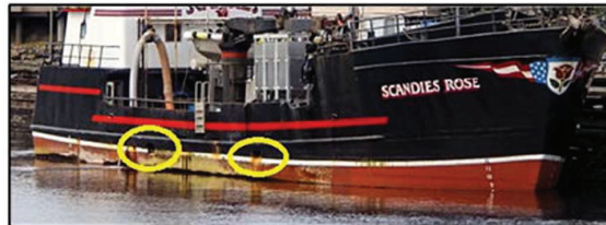
Figure 33 - Starboard side of the SCANDIES ROSE prior to the repair of the overboard chutes, taken several years earlier. Yellow circles indicate two chutes, one forward and one aft through the side shell plating and into the starboard pipe alley. (Source Mr. [REDACTED] ©, with permission and with Coast Guard mark up)
