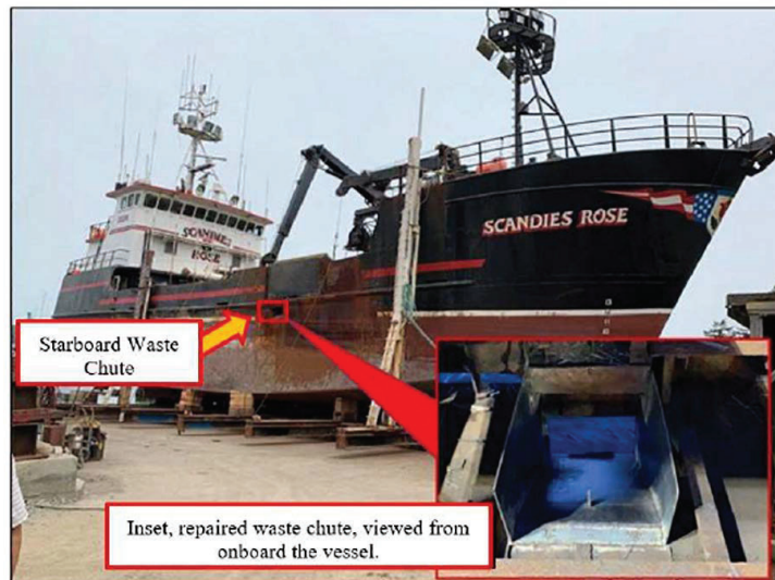
Figure 34 – SCANDIES ROSE on the blocks May 2019 at Lovric’s Shipyard, Anacortes, WA. “Starboard Waste Chute” highlighted, inset photo, lower right, displays the completely rebuilt starboard waste chute as repaired later in 2019 by High Mark Marine certified welders. (Source [REDACTED], with Coast Guard mark up)
