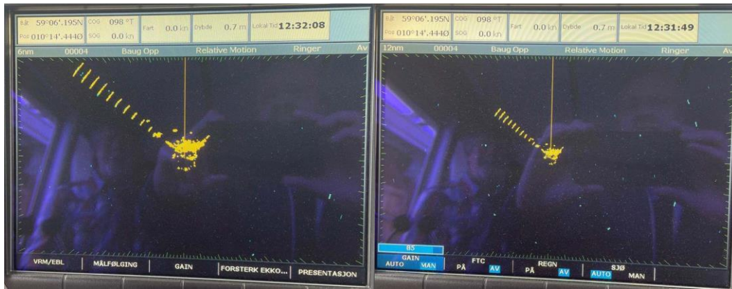
Figure 9. The radar's display at "position A." Note one image shows the radar display's range rings set to 6 NM, and the other to 12 NM.
