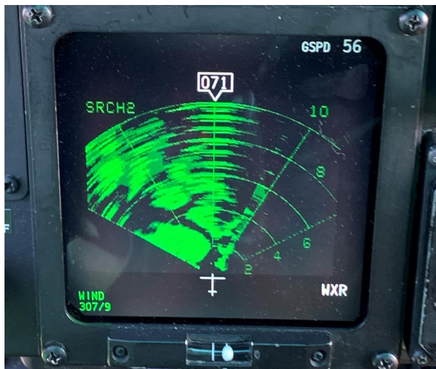
Figure 15. A picture of the MH-65C's RDR-1300C radar display when receiving the SART.
