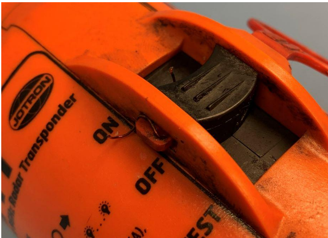
Figure 2. Broken safety wire (copper color) indicating the device had been activated at some time.
