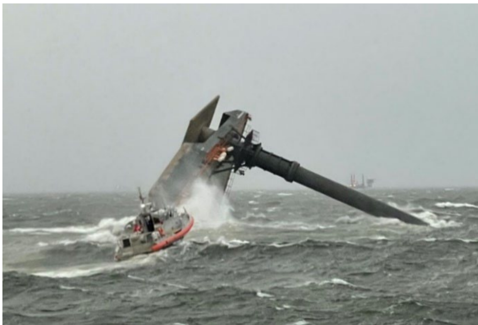
Figure 8. SEACOR Power capsized on its starboard side on the evening of the casualty, with a Coast Guard RB-M in the foreground and the liftboat Rockfish in the background. (Source: Coast Guard)
