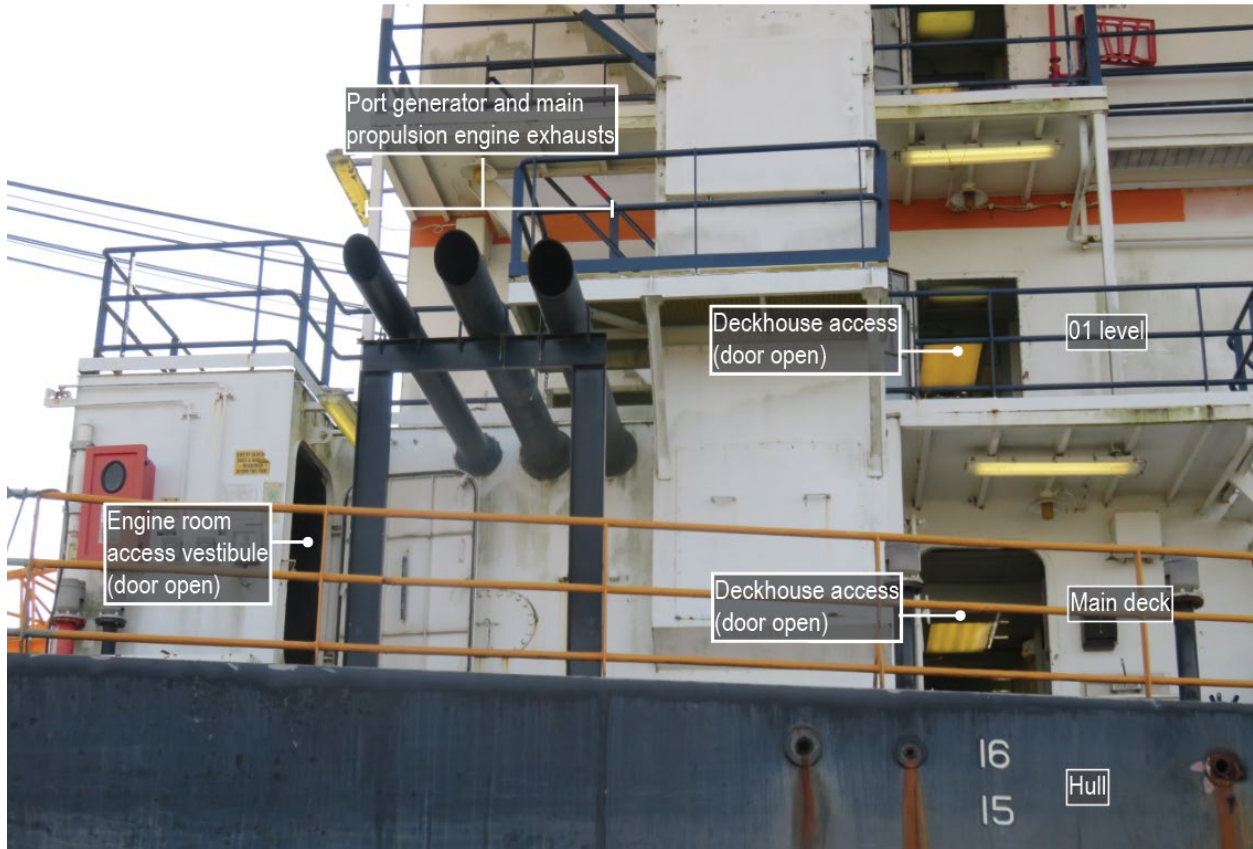
Figure 12. Portside deckhouse and engine room accesses on similar vessel SEACOR Legacy .
